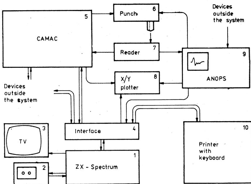
Fig. 1. Block diagram of the system. Arrows indicate directions of possible data transmission. For further description see text.
